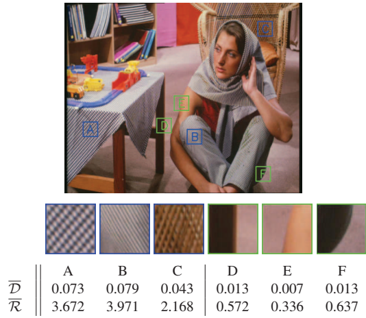
Figure 2: Local variation deviation for different patches. \overline{D} and \overline{R} are the averages of variation deviation in the local patches. The local variation deviation provides strong discriminative power in distinguishing texture (in blue bounding box) and structure (in green bounding box).
